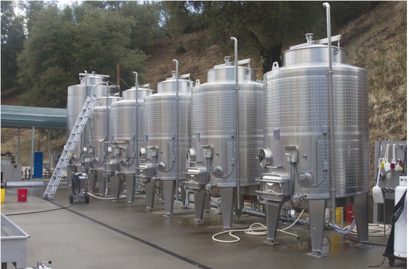
Six Sigma Ranch now has 12 stainless steel tanks for wine fermentation, double the number the fledgling business began production with in 2005. From any laptop computer, the winemaking team can monitor and manipulate critical-to-quality attributes within the tanks.
